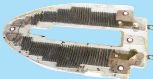
Fig. 14.11 Element of electric iron
