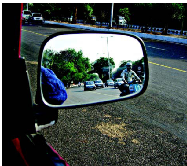
Fig. 15.20 Convex mirror as side view mirror
